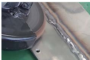
Removing blue weld discoloration
