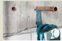
Copper pie flush cutting
