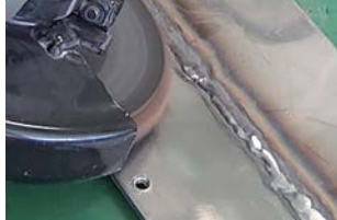
Removing blue weld discoloration
