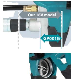
Shorter grease path reduces air lock during cartridge replacement.
