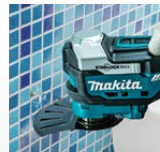
Routing joints on wall tiles
