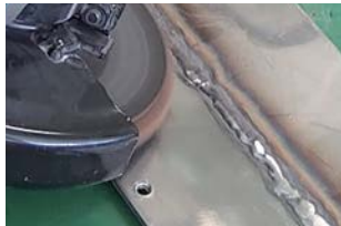
Removing blue weld discoloration
