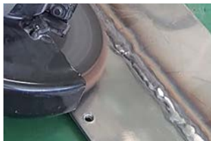
Removing blue weld discoloration
