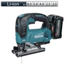
Capacity Wood: 135 mm (5-5/16") Mild Steel: 10 mm (3/8") Aluminum: 20 mm (25/32") Stroke length 26 mm (1") 0 - 3,500 0 - 45° Strokes per minute (S Bevel range Woodwork: 6 1m/s2 Vibration level Metalwork: 4.2m/s<sup>2</sup> Dimensions w/BL4025: 272×84×208mm Net weight 2.6 kg (5.7 lbs.)
