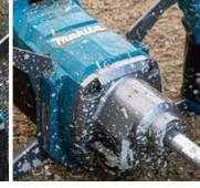
Switch cover is minimizes the chance that switch trigger or lock-on button might be stuck by adhered and hardened material.
