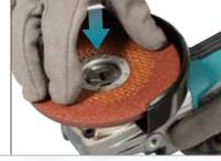
Just one click to attach the accessories easy removal just simply pull the lever
