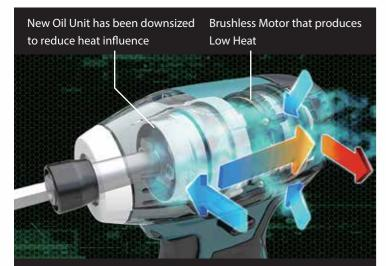
Rear fan efficiently cools down Oil Unit & Motor
