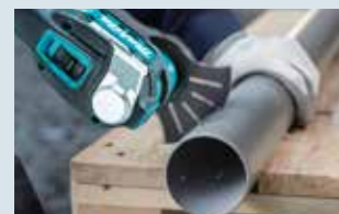
Cutting PVC, FRP pipes
