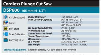
The weight may differ depending on the attachment(s), including the battery cartridge.
