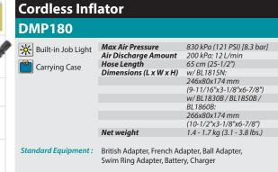
The weight may differ depending on the attachment(s), including the battery cartridge. The lightest and heaviest combination, according to EPTA-Procedure 01/2014, are shown in the table.
