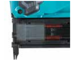
with window for check of remaining nails.
